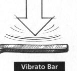
The Vibrato Bar is made from <sup>3</sup>/<sub>16</sub> hexagonal stainless steel. This special alloy can be bent to your liking and will retain its shape in use. We recommend that you let a guitar
